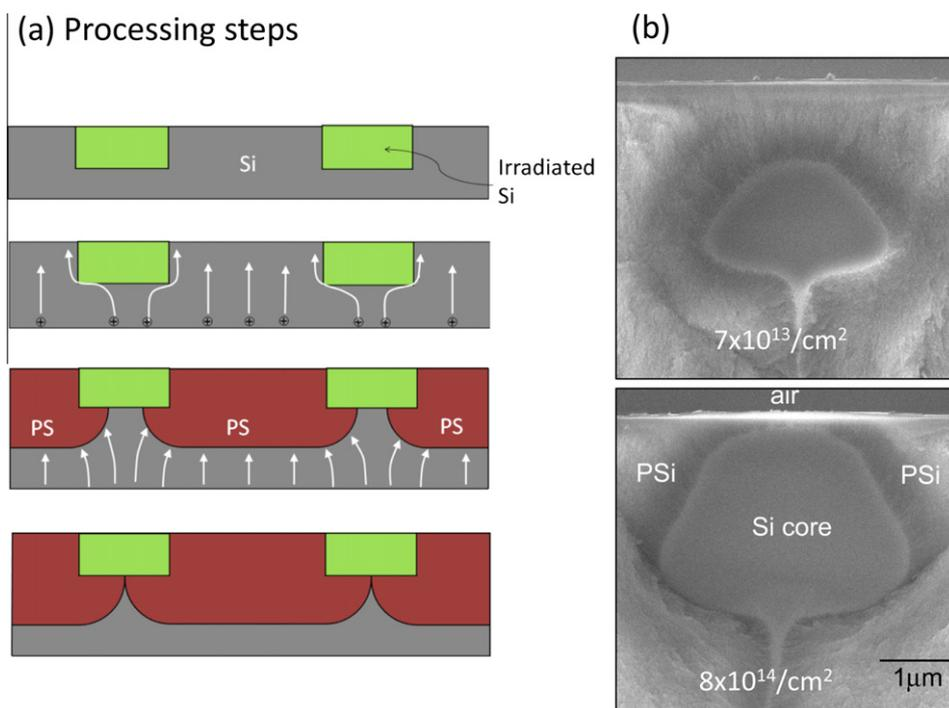
**Fig. 1.** (a) Schematic fabrication process for waveguide fabrication (b) Cross sectional SEM of the channel waveguides irradiated with 250 keV protons at fluencies of 7 and  $8 \times 10^{14}/\text{cm}^2$ .
