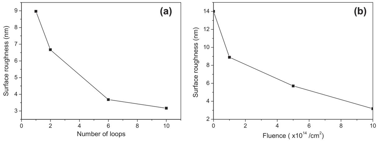
Fig. 2. (a) Plot of surface roughness vs number of loops and (b) ion fluence.
