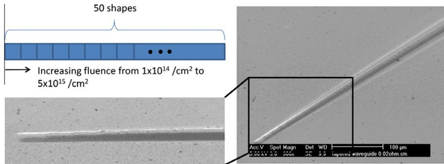
Fig. 3. Irradiation of a taper profile with fluence linearly increasing from  $1 \times 10^{14} / \text{cm}^2$  to  $1 \times 10^{15} / \text{cm}^2$  (from left to right). Also shown are the SEM images of the tapered profile.
