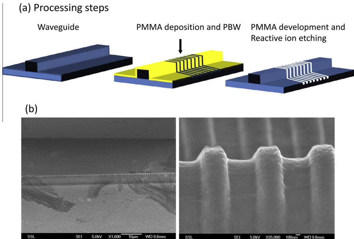
Fig. 4. (a) Schematic diagram of the processing steps. (b) SEM images of a waveguide grating.
