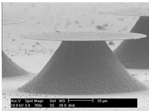
Fig. 5. SEM image of a 200 nm thick silicon disk resonator supported on a pedestal.
