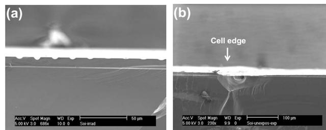
**Figure 4.** Cross-section SEMs of the ac anodized SOI wafer close to the cell edge. (a) The nonuniform lateral anodization. (b) The deep groove forming at the cell edge.
