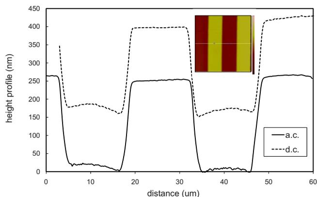
**Figure 2.** (Color online) AFM line profiles 10  $\Omega$  cm p-type bulk silicon anodized in ac and dc modes, offset for clarity. The inset shows a  $60 \times 60 \mu\text{m}$  AFM image of the ac anodized wafer surface.
