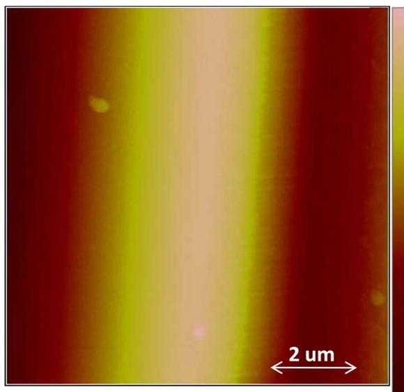
**Figure 5.** (Color online) AFM image of a single irradiated line in SOI after ac anodization using a line focus of 2 MeV protons.
