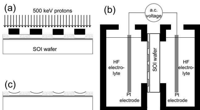
**Figure 1.** Schematic of the ac anodization process. (a) Proton irradiation through a thick patterned PMMA layer (shown in black) results in a patterned SOI device layer. (b) Teflon cell (shown in black) for ac anodization of SOI wafer. (c) Removal of porous silicon producing a patterned SOI device layer.
