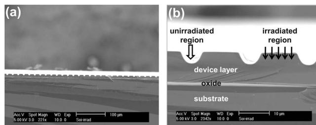
**Figure 3.** Cross-section SEMs of the central portion of the ac anodized SOI wafer at different magnifications.
