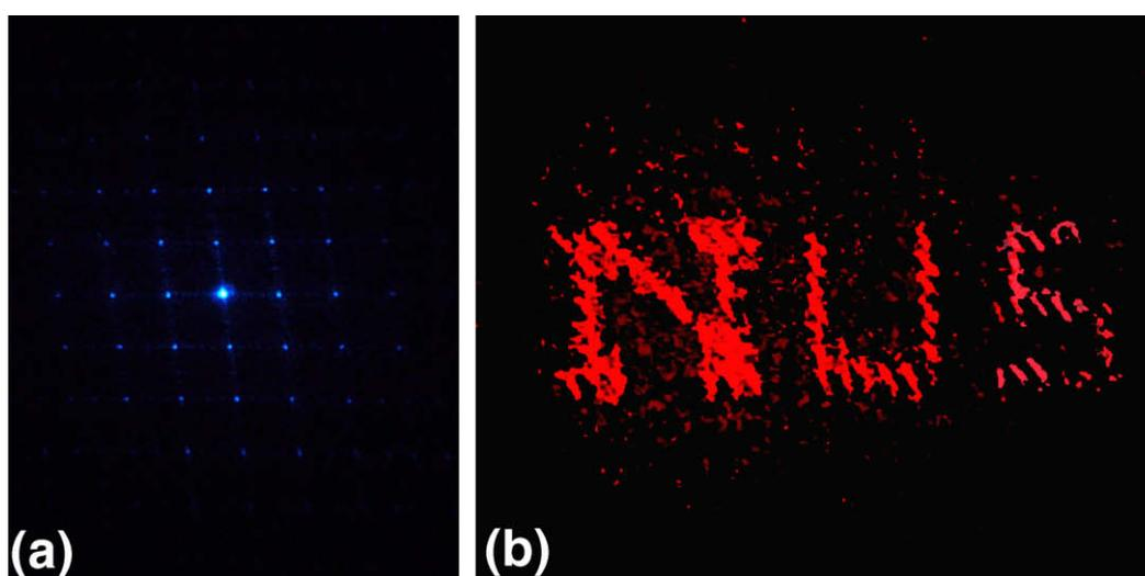
Fig. 4. (a) Diffraction pattern, and (b) reconstructed holographic image of NUS CGH pattern.
