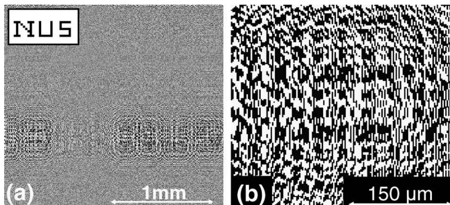
Fig. 2. (a) Inset shows NUS input file, comprising 30 by 15 pixels. (a) and (b) Corresponding CGH pattern at different magnifications.
