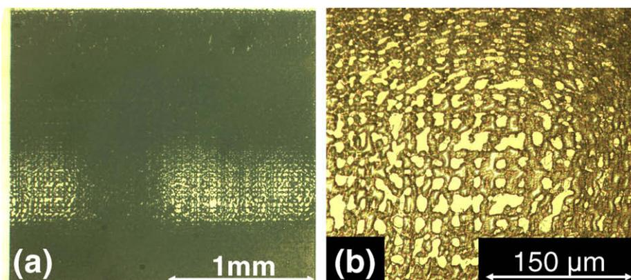
Fig. 3. The developed PMMA structures of the CGH pattern shown in Fig. 2.
