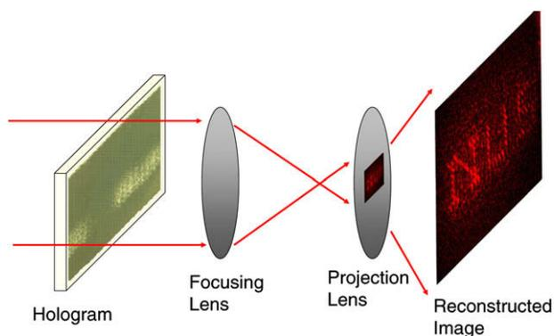
Fig. 1. Schematic of holographic reconstruction set-up.
