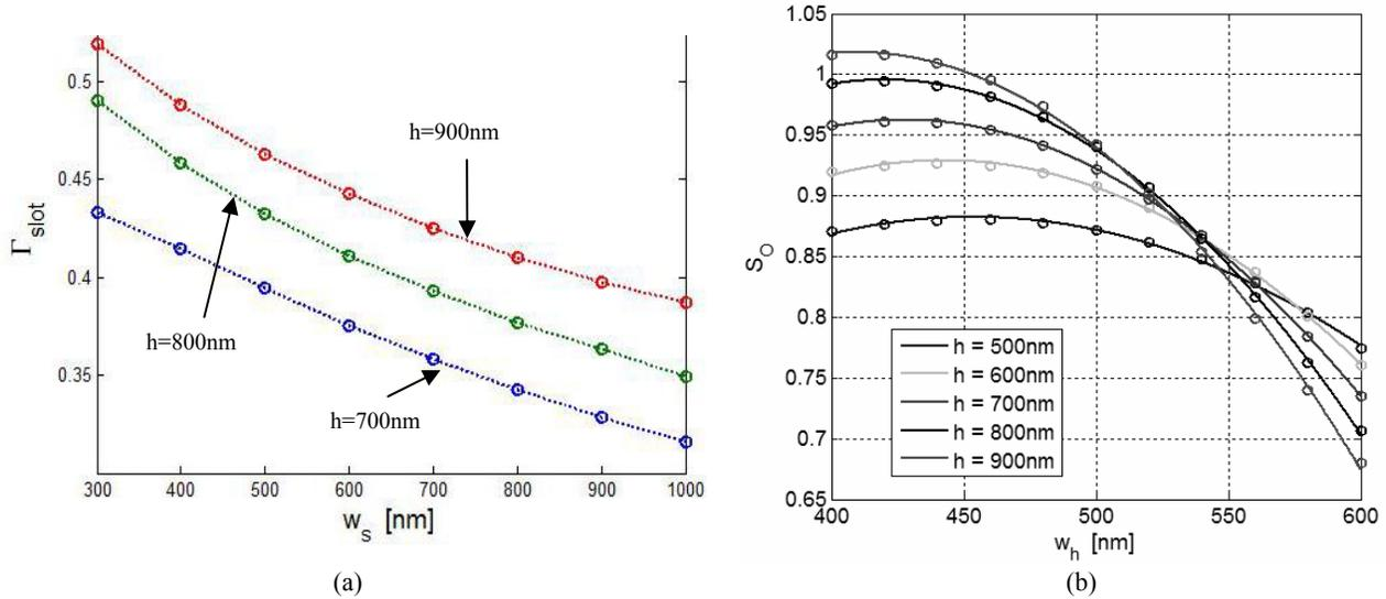
Fig. 5: (a) Maximum confinement factor of quasi-TE mode as a function of slot width  $w_s$  and height  $h$  for an air cover; (b) Sensitivity to the slot refractive index change versus wire width  $w_h$  and for different heights  $h$  ( $w_s=400$  nm)
