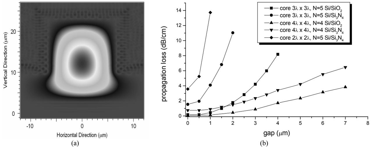
Fig. 2: (a) Mode profile for a hollow waveguide with Si/Si<sub>3</sub>N<sub>4</sub> Bragg reflectors and a gap between the two reflectors; (b) Propagation loss of hollow waveguides with Si/SiO<sub>2</sub> and Si/Si<sub>3</sub>N<sub>4</sub> Bragg reflectors as a function of the gap between the two claddings
