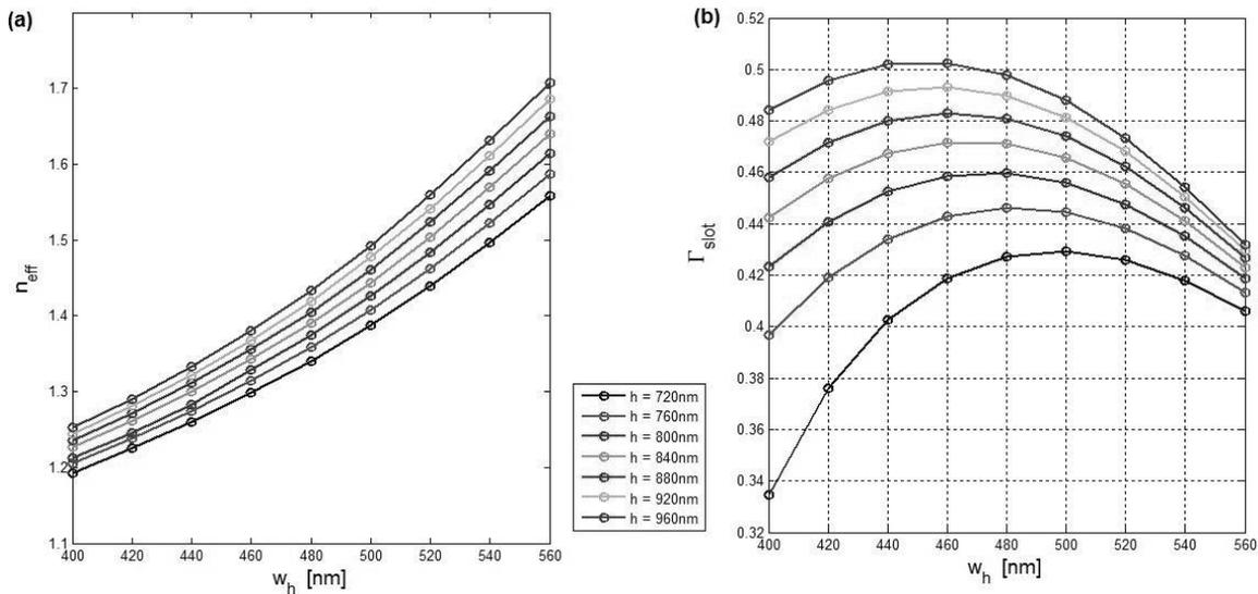
Fig. 4: (a) The effective index and (b) the slot confinement factor for the quasi-TE mode in the slot with air cover as a function of the silicon wire width  $w_h$  and height  $h$  (slot width  $w_s = 400$ nm)
