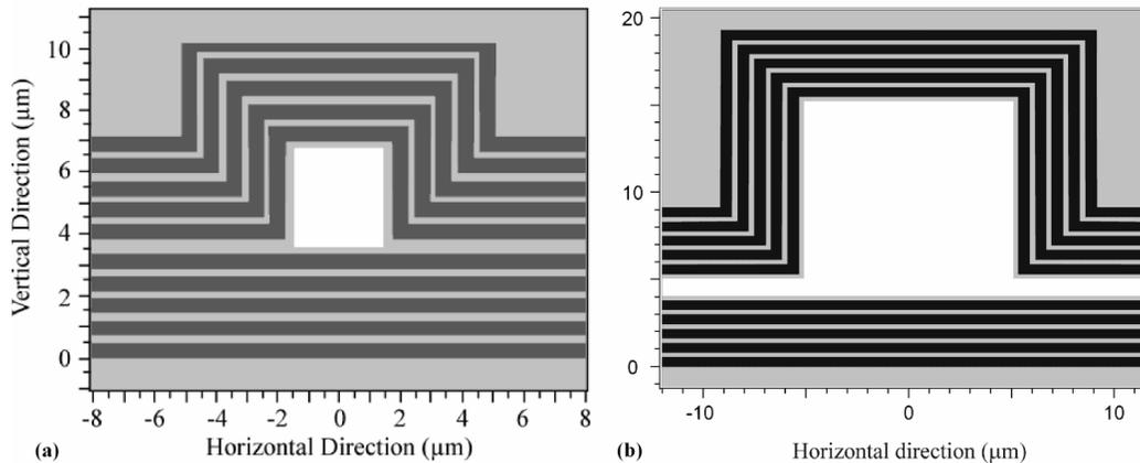
Fig. 1: Bragg type hollow waveguide a) without a gap between the two bonded wafers, b) with the gap
