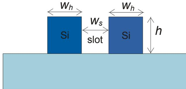
Fig. 3: Schematic of the slot waveguide
