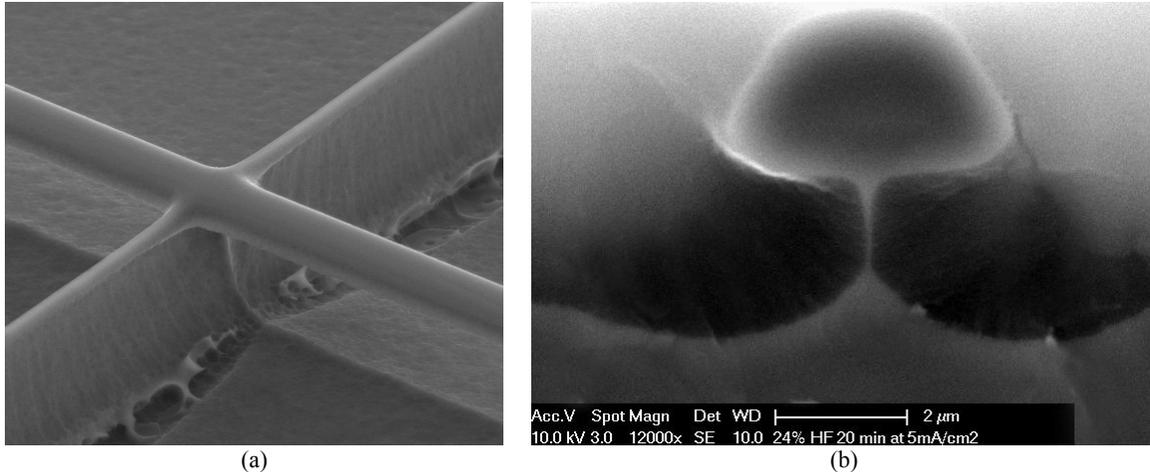
Fig. 6: a) SEM micrograph of a free-standing waveguide b) cross sectional SEM view of a waveguide with porous Si cladding
