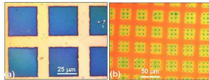
Fig. 2. Large area patterned DBRs produced by irradiation with 750 keV He ions with free-standing nickel grids placed over the wafer surface. (a) formed using a single 50  $\mu\text{m}$  period grid, (b) with an additional 12.7  $\mu\text{m}$  period grid.
