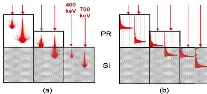
Fig. 3. SRIM plots of 400 and 700 keV  $\text{H}_2^+$  ions incident on different thicknesses of PR on top of a  $7\text{-}\mu\text{m}$  thick Si layer (shown in gray). From left to right the PR thicknesses are  $7\mu\text{m}$ ,  $3\mu\text{m}$  and 0 (a) trajectory plots showing how far each ion penetrates through the layer structure. (b) defect density in each case. Both beam energies are shown, with the higher energy to the right
