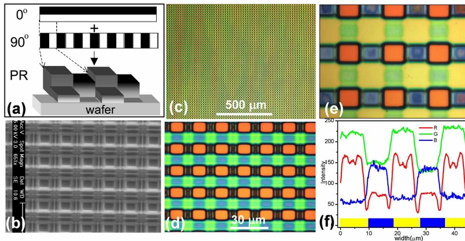
Fig. 5. (a). Schematic of the fabrication procedure to produce multilevel square pixels in the PR. (b) SEM of the PR pixels with different thicknesses on the wafer surface. (c), (d) high and low magnification optical reflective images of the patterned DBR. (e) optical reflective image of the patterned RYGB pixels. (f) line scan of reflected intensity across the yellow and blue pixels.
