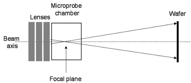
Fig 1. Schematic of microprobe ion optical system used to project a large area, uniform intensity of beam over wafer surface which is located downstream of the chamber.
