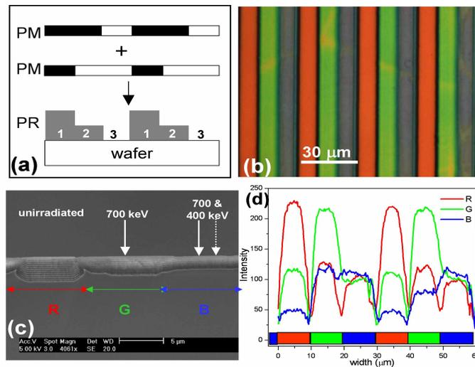
Fig 4. (a). Schematic of two photomasks (PM) used to create a multilevel photoresist (PR) mask on the wafer surface. (b) optical reflective images of 10 μm wide DBR lines in three different colours. (c) XSEM view of the DBR layers formed across the RGB lines in (b). (d) horizontal line scans showing the intensity of red, green and blue across the patterned DBR structure.
