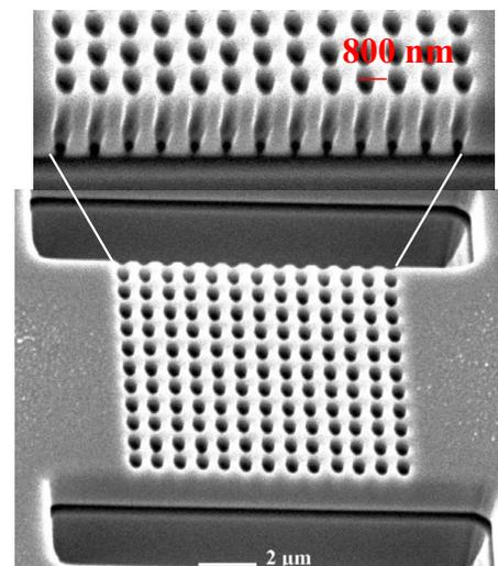
FIG. 6. (Color online) Fabricated PCs in a suspended slab. The holes have been milled through the slab.
