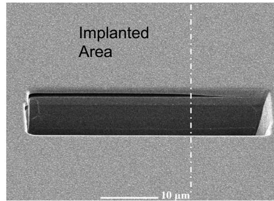
FIG. 3. SEM image of a rectangular hole patterned on the edge of the implanted area.
