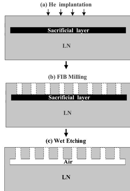
FIG. 1. Illustration of the process steps to create suspended structures in LN using ion implantation, FIB milling, and selective wet etching.
