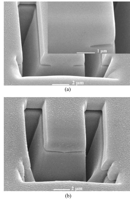
FIG. 5. Cross-sectional images showing the undercut after (a) 10 min and (b) 20 min of wet etching. The inset in (a) shows a further magnified view of the right undercut structure.
