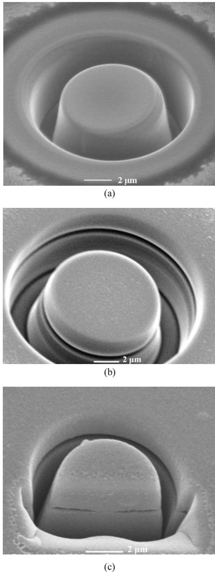
FIG. 4. (a) FIB image of a post after milling and before wet etching. (b) SEM image of a post after wet etching. (c) SEM image showing the cross-sectional view.
