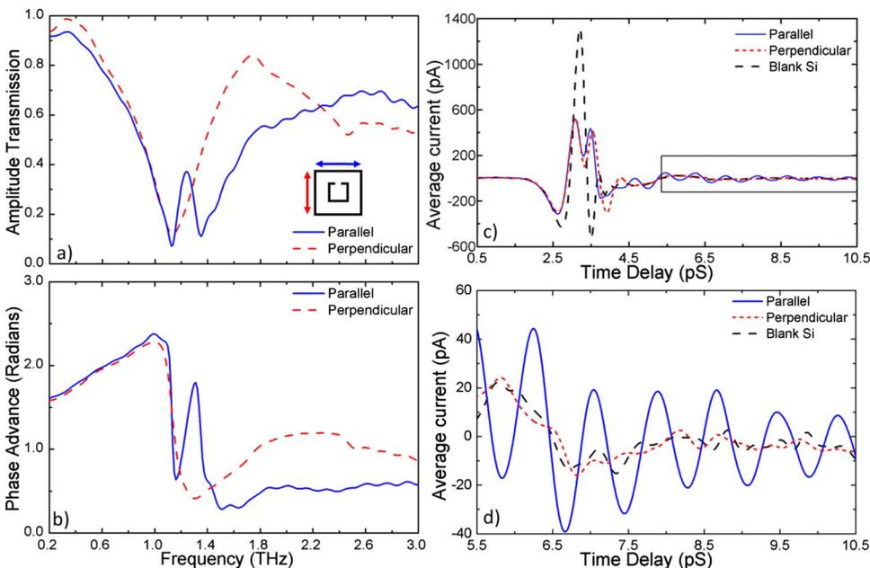
FIG. 2. (Color online) (a) Measured amplitude transmission and (b) phase advance for the fabricated sample as a function of frequency and for two polarization states of the illumination. Insets show the orientation of the  $E$  field for parallel (blue, solid) and perpendicular (red, dashed) polarization. The measured data in time domain are shown in (c) where the slowly decaying oscillations at  $1.25 \text{ THz}$  under parallel polarization in the marked area are zoomed in (d).
