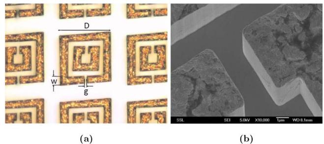
FIG. 1. (Color online) Optical (a) and scanning electron (b) micrographs of the gold SRRs fabricated for this work. The dimensions of the SRR are approximately  $D=38 \mu\text{m}$ ,  $w=6 \mu\text{m}$ , and  $g=2 \mu\text{m}$ . The unit cell length is 50  $\mu\text{m}$ .
