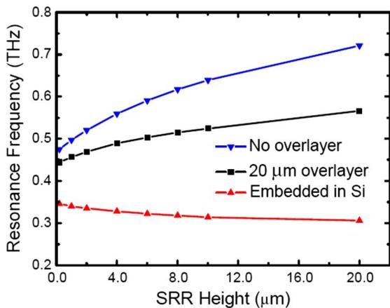
FIG. 4. (Color online) Plot of simulated  $\omega_{LC}$  for SRRs without (blue curve) and with (black curve) a 20  $\mu\text{m}$  dielectric overlayer. For SRRs, completely embedded in Si (red curve), the trend is reversed.
