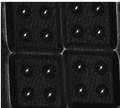
Fig. 4(a). View of the focal plane of the microlens array of diameter 150 μm, showing uniform arrays of focal points. It is a measure of the quality of replicated microlens array.
