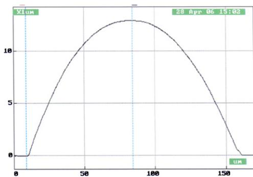
Fig. 3. Line profilometer measurement of one of the replicated microlenses out of an array of microlens of 150 μm diameter. The horizontal direction represents diameter of a microlens, and the vertical direction represents the height of the lens.
