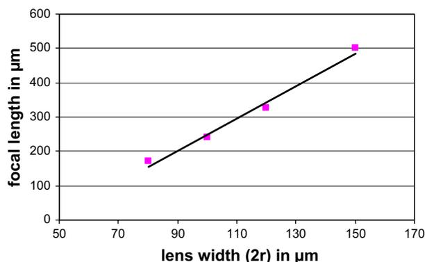
Fig. 5. A plot showing linear relationship between width of microlens (aperture) in x-axis vs. measured focal length in y-axis. The linearly drawn line represents the expected focal length against its corresponding aperture of the lens. The dots are experimentally measured values of focal length with respect to its corresponding aperture of microlens.
