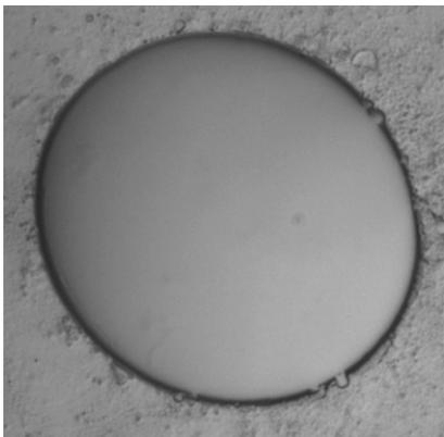
Fig. 2(b). Zoomed image of a replicated microlens (as marked by a box in Fig. 2(a)) showing details of the structure.
