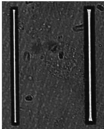
Fig. 4(b). View of the focal plane of cylindrical microlens of 70 μm width (the left of the fig). Note that the cylindrical lens on the right is out of focus as its width is 100 μm.
