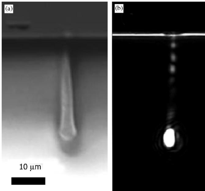
Fig. 2. Optical images of a waveguide fabricated in PMMA using a beam of 2.0 MeV protons. (a) DIC optical image of the edge of a PMMA waveguide sample showing the end of range region. (b) Optical image of a guided mode (HeNe—632.8 nm laser) in the same sample. A fluence of  $2.2 \times 10^{13}$  protons/cm<sup>2</sup> was used to fabricate this waveguide.
