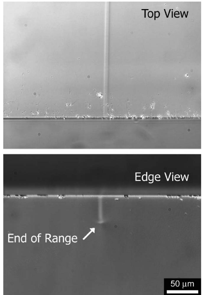
Fig. 3. Optical DIC images showing a waveguide fabricated in Foturan photosensitive glass using a beam of 2.0 MeV protons and a fluence of  $1 \times 10^{16}$  protons/cm<sup>2</sup>. The side view of the sample clearly shows the end of range region.
