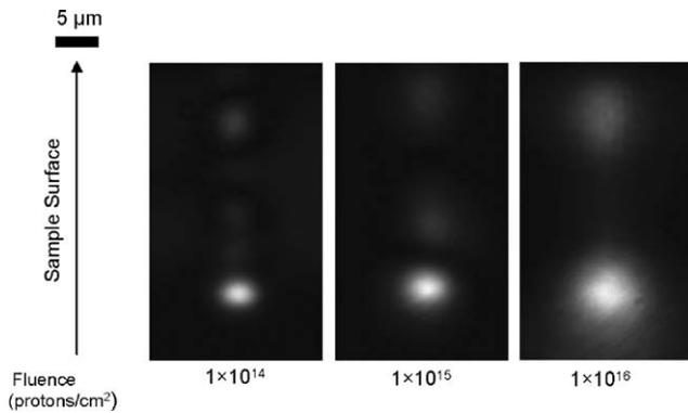
Fig. 4. Optical images in pseudo-color showing the modes supported by three waveguides fabricated in Foturan glass. The modes are shown for three different proton fluences.
