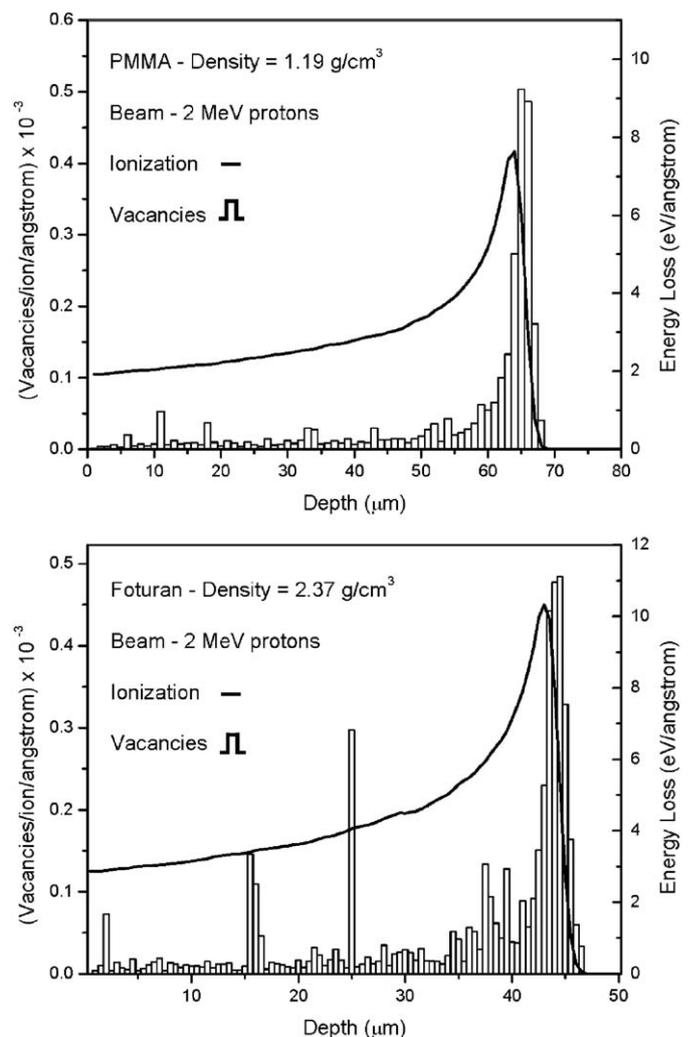
Fig. 1. SRIM simulation of the ionization and vacancy profile produced by a beam of 2.0 MeV protons in PMMA and Foturan.
