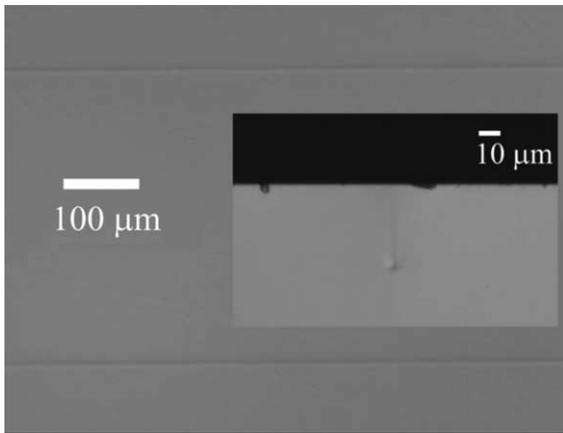
Fig. 2. Differential interference contrast (DIC) image of the top-view of a pair of proton beam written waveguides. Inset shows a DIC image of the end-face of one of the waveguides.
