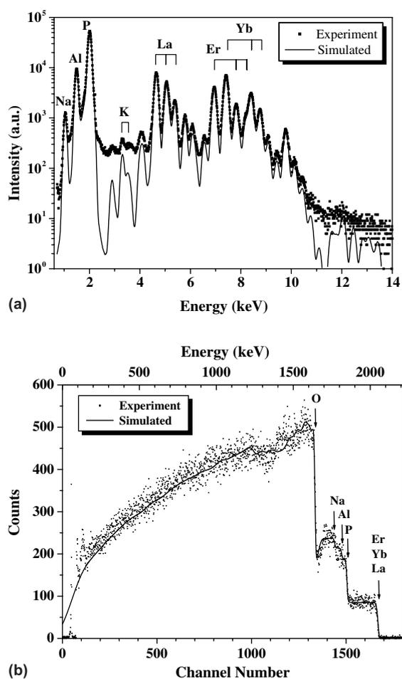
Fig. 1. (a) PIXE spectrum of the IOG-1 glass sample (co-doped with 2.16 wt% of  $\text{Er}_2\text{O}_3$  and 4.70 wt% of  $\text{Yb}_2\text{O}_3$ ), (b) RBS spectrum of the sample.
