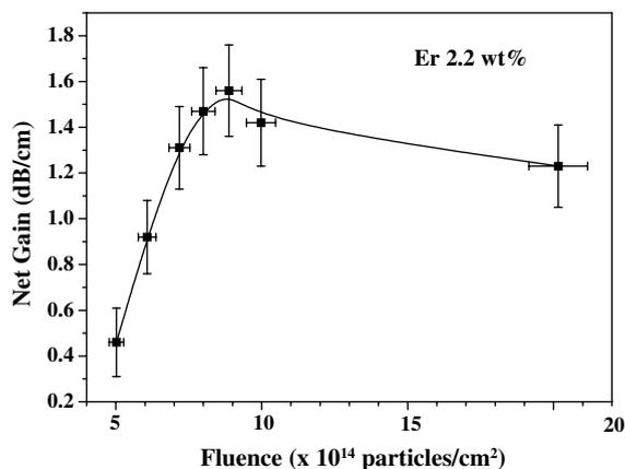
Fig. 5. Graph of net optical gain against the proton fluence used in the fabrication.
