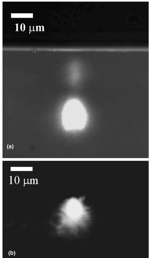
Fig. 4. Near-field mode profiles of a waveguide fabricated with a fluence of  $1 \times 10^{15}$  particles/cm<sup>2</sup> at a wavelength of (a) 632.8 nm and (b) 1550 nm.
