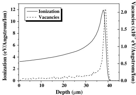
Fig. 3. TRIM simulation results for 2.0 MeV protons in IOG-1 phosphate glass.
