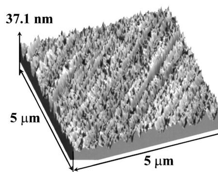
FIG. 2. A 3D AFM image of the sidewall morphology over a  $5 \times 5 \mu\text{m}^2$  scan area. Structure was fabricated using a scanning speed of  $\sim 10 \mu\text{m/s}$ .
