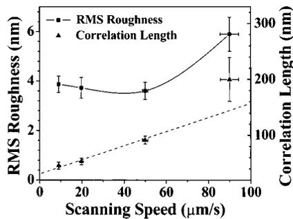
FIG. 4. A plot of the rms roughness (■) and a linear fit of the correlation lengths (▲) as a function of the stage scanning speeds.
