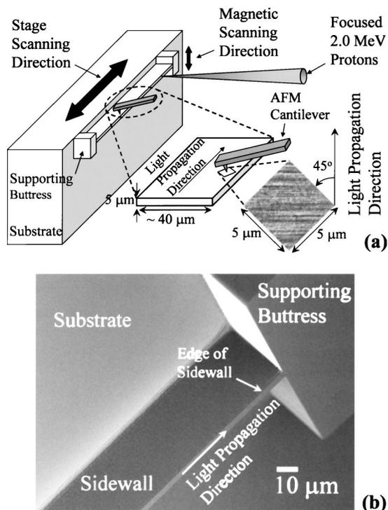
FIG. 1. (a) A schematic of the proton beam written structure and a typical AFM image of its sidewall morphology. The relative orientations of the magnetic and stage scanning directions used in the proton beam writing are indicated. (b) A SEM image of the fabricated structure.
