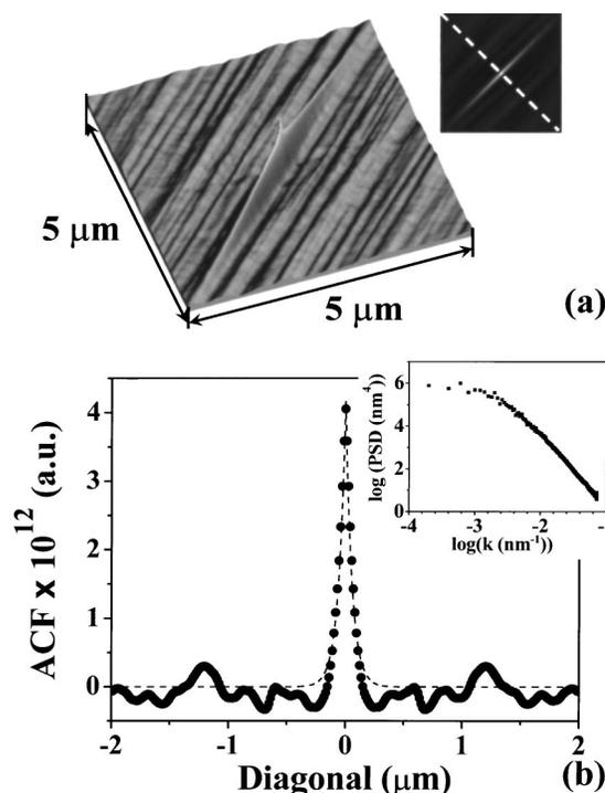
FIG. 3. (a) A 3D view of the 2D ACF of the AFM surface shown in Fig. 2. The inset shows a planar 2D view of the same function. (b) An exponential fit of the extracted 1D ACF (i.e., extracted diagonally across the 2D ACF, orthogonal to the undulations as indicated by the dotted diagonal line in (a) inset). The inset shows the corresponding power spectral density function.
