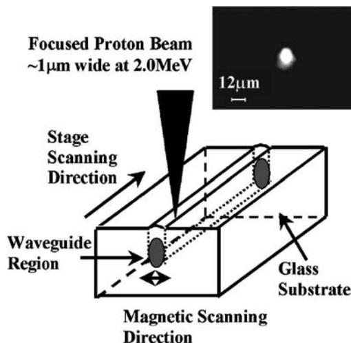
FIG. 1. Schematic diagram of the focused PBW fabrication process. A combination of stage scanning and magnetic scanning was used to write the waveguides.
