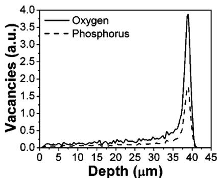
FIG. 3. Distribution of oxygen and phosphorus vacancies in phosphate glasses as a function of the penetration depth using TRIM simulation. The proton energy used is 2.0 MeV.
