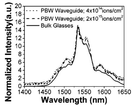
FIG. 4. Fluorescence and ASE spectra of bulk glasses and PBW waveguides.
