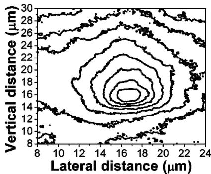
FIG. 2. Contour plots at the end face of a PBW waveguide (ion dose  $\sim 2 \times 10^{15}$  ions/cm<sup>2</sup>). Eight contour levels are used, and each is spaced  $\sim 2.9$  nm.
