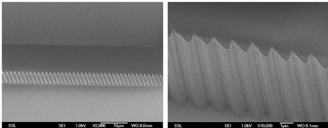
Fig. 3. SEM images of a blazed grating micromachined in a 10 μm layer of SU-8 on a Si substrate.
