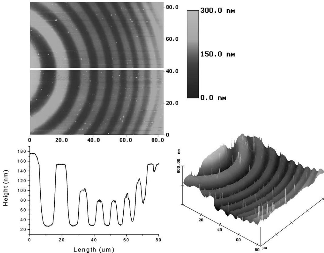
Fig. 6. AFM image of a section of one of the micro-Fresnel lens elements in Fig. 5. A line scan showing the surface compaction is also shown.
