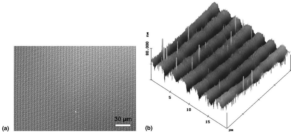
Fig. 2. (a) Differential interference contrast (DIC) optical image of an implanted line grating in PMMA. (b) AFM image of a section of the same grating structure. The PMMA sample is modified using 2 MeV protons and a dose of 100 nC/mm<sup>2</sup>.
