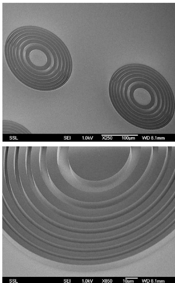
Fig. 4. SEM images of some micro-Fresnel lens elements micro-machined in a 10  $\mu\text{m}$  layer of SU-8 on a Si.
