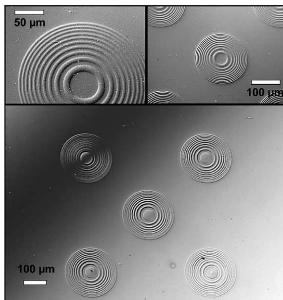
Fig. 5. DIC images of some micro-Fresnel lens elements micro-machined in a bulk PMMA sample.
