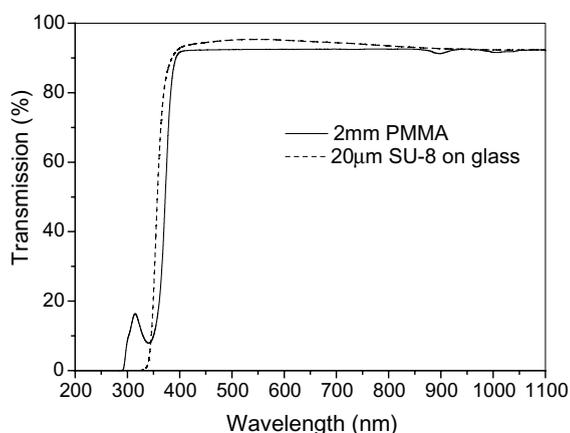
Fig. 1. Optical transmission spectrum measured from a 2 mm thick sample of PMMA and a 20 μm unexposed layer of SU-8 spin coated on a glass substrate.
