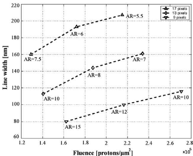
Fig. 5. Measured widths (average) of different lines written with 2 MeV protons in  $1.2 \mu\text{m}$  thick HSQ on Cr/Si and Ti/Si substrates as function of the proton fluence. The aspect ratio (AR) is given for every line.
