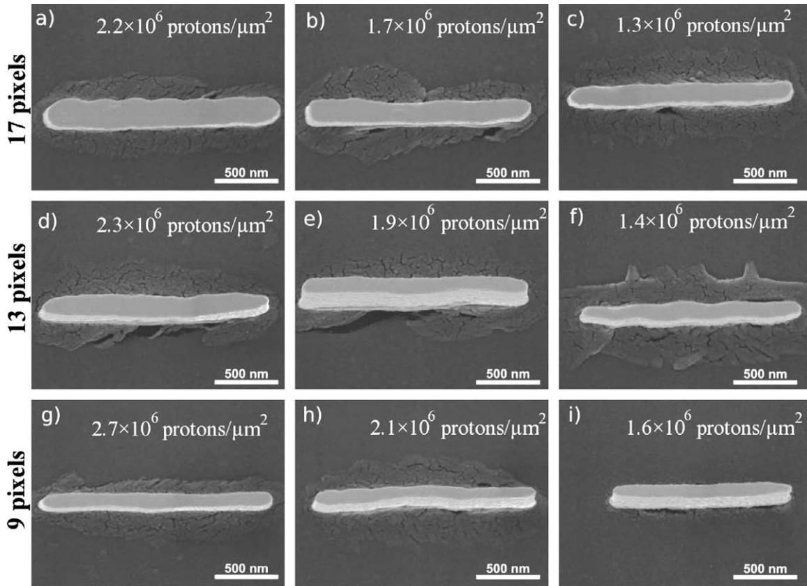
Fig. 3. Lines of different width written with 2 MeV protons in 1.2  $\mu\text{m}$  thick HSQ on a Cr/Si substrate.
