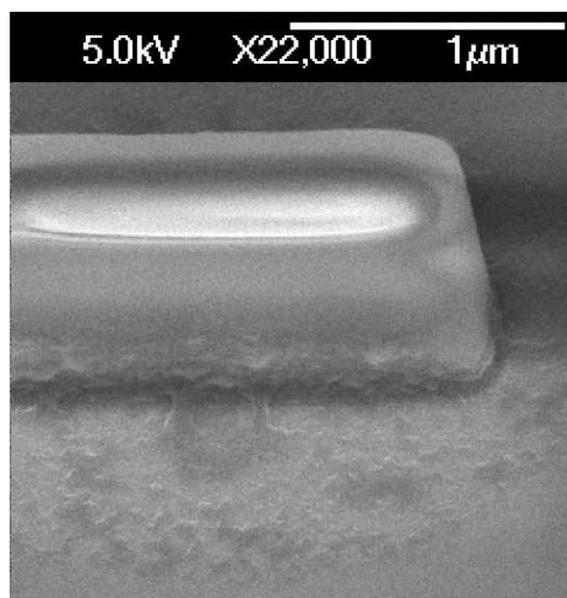
Fig. 2. “Halo”-like grainy structures around lines written on a Cr/Si substrate.
