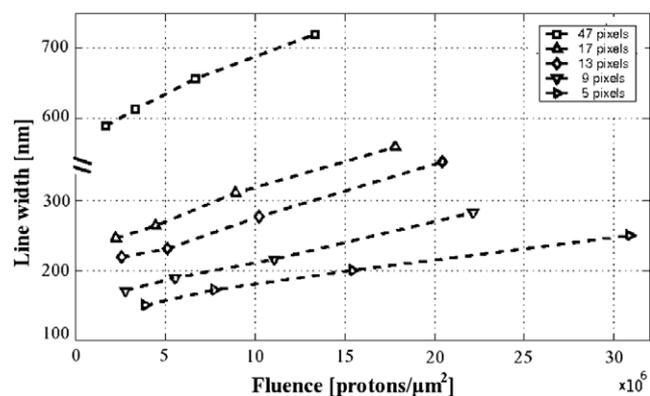
Fig. 1. Measured widths of different lines written with 2 MeV protons in 1.2  $\mu\text{m}$  thick HSQ on Cr/Si, Ti/Si and Au/Cr/Si substrates as function of the proton fluence.
