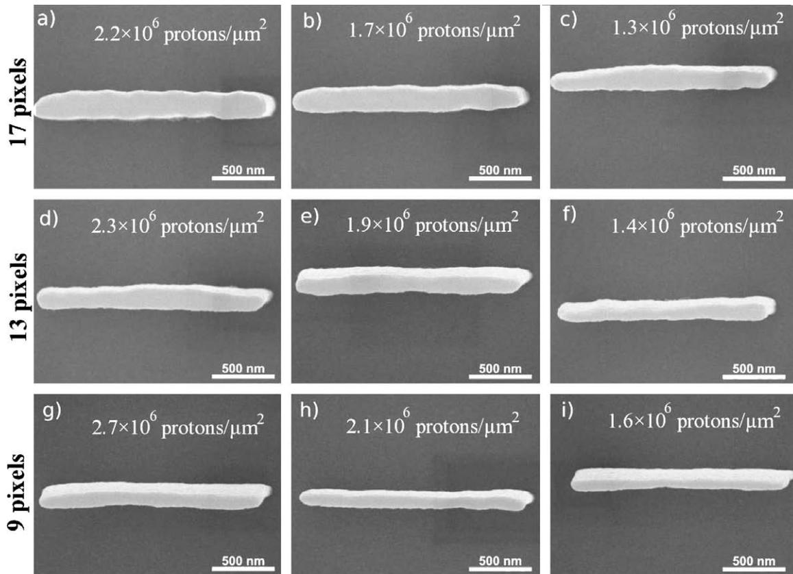
Fig. 4. Lines of different width written with 2 MeV protons in 1.2  $\mu\text{m}$  thick HSQ on a Ti/Si substrate.
