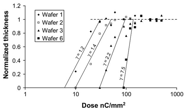
Fig. 2. Contrast curve for wafers 1, 2, 3 and 6 for 2 MeV proton exposure. The thickness is normalized to one, for fully crosslinked resist.
