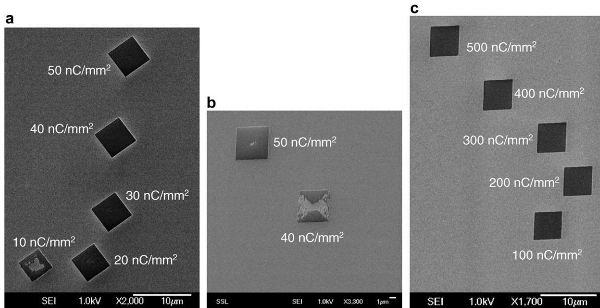
Fig. 1. SEM images of  $5 \times 5 \mu\text{m}^2$  squares written with a 2 MeV proton beam: (a) exposed in wafer 1 with 10–50 nC/mm<sup>2</sup>, (b) exposed in wafer 3 with 40 and 50 nC/mm<sup>2</sup> and (c) exposed in wafer 6 with 100–500 nC/mm<sup>2</sup>.
