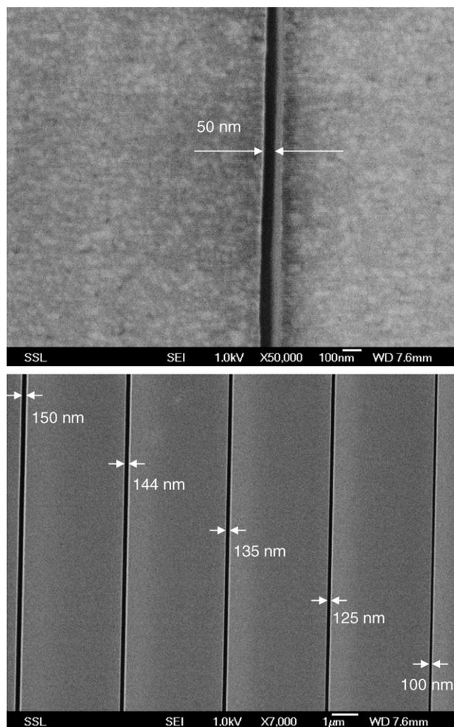
Fig. 3. SEM images of narrow lines exposed in wafer 1 (coated in 2005 and exposed in 2007), featuring 150 down to 50 nm wide lines exposed with 2 MeV protons in 850 nm thick HSQ resist.
