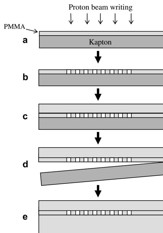
Fig. 1. Schematic representation of the process of the enclosed channel fabrication using proton beam writing.
