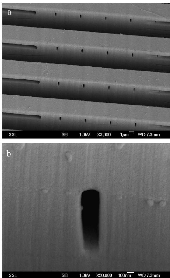
Fig. 3. (a) PMMA enclosed nanochannels fabricated using proton beam writing coupled with thermal bonding, and (b) close up of one of the buried channels. The channels are 200 nm wide and 2  $\mu\text{m}$  deep.
