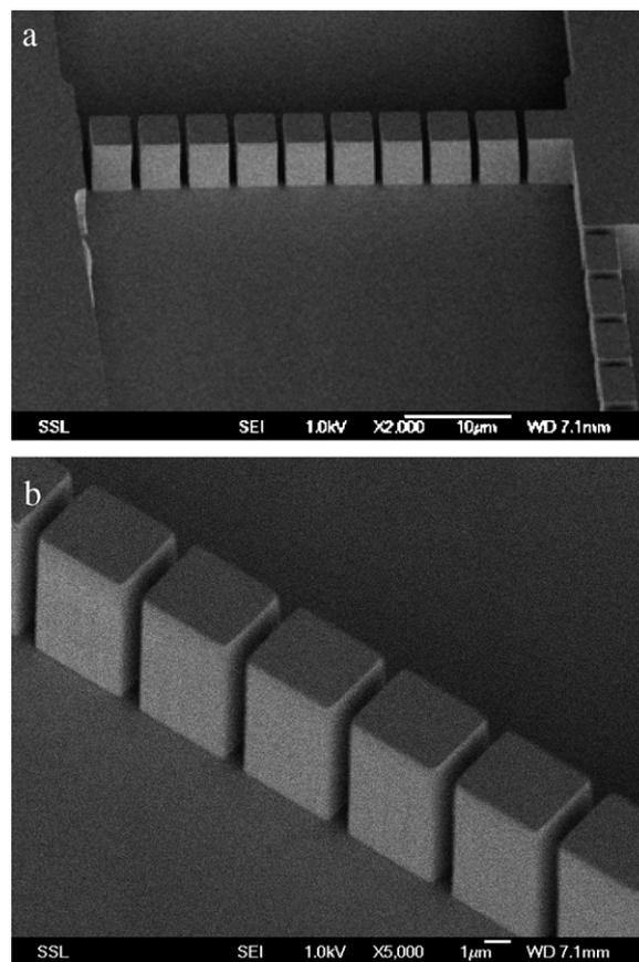
Fig. 2. (a) PMMA micropillars transferred to bulk PMMA from a Kapton substrate, (b) high resolution image of (a). The grooves are 800 nm wide.
