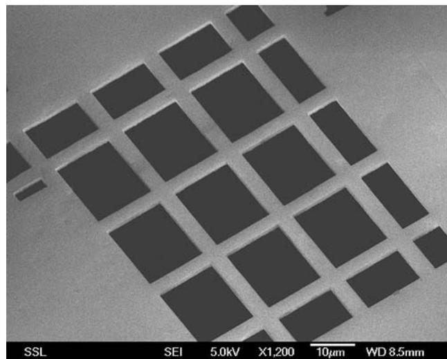
**Fig. 4** SEM of 2  $\mu\text{m}$  thick Ni stencil mask produced by p-beam writing in a 3  $\mu\text{m}$  PMMA layer followed by Ni electroplating
