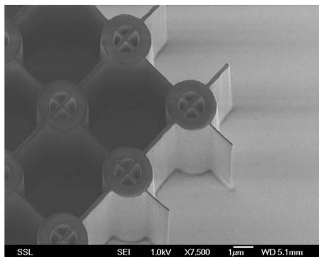
Fig 2 SEM of p-beam written high aspect ratio structures in 10  $\mu\text{m}$  thick SU-8 featuring 60 nm walls
