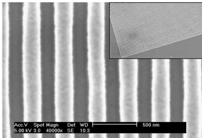
**Fig. 3** SEM of a Ni stamp featuring 180 nm lines and spaces, 200 nm deep, the stamp has a total thickness of 1.1 mm. The inset shows an overview of the grating
