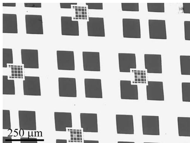
**Fig. 5** Optical photograph of a 20  $\mu\text{m}$  thick Ni stencil mask produced by p-beam writing in a 25  $\mu\text{m}$  PMMA layer followed by Ni electroplating
