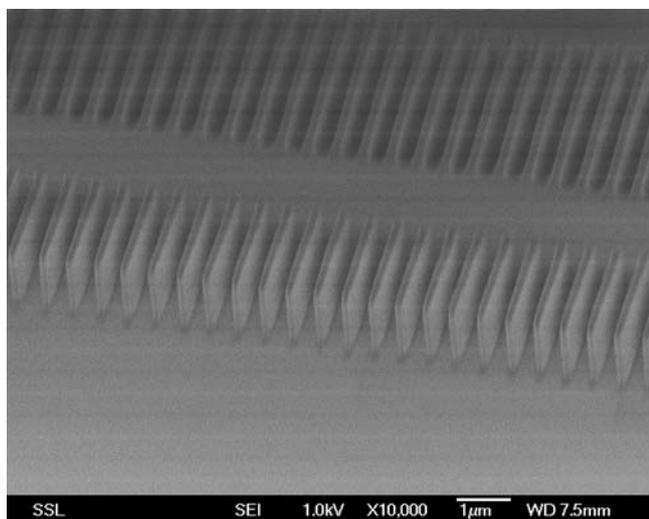
Fig. 1 SEM of p-beam written 130 nm lines in 2  $\mu\text{m}$  thick SU-8
