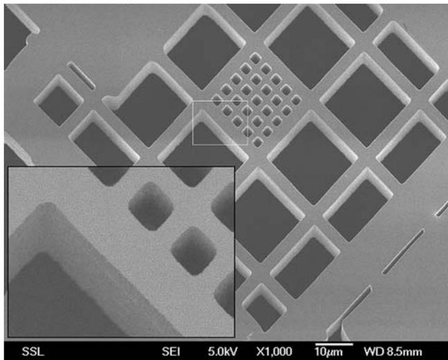
**Fig. 6** SEM of the 20  $\mu\text{m}$  thick Ni stencil mask featuring 1  $\mu\text{m}$  details and an aspect ratio of 20. The inset shows the marked area
