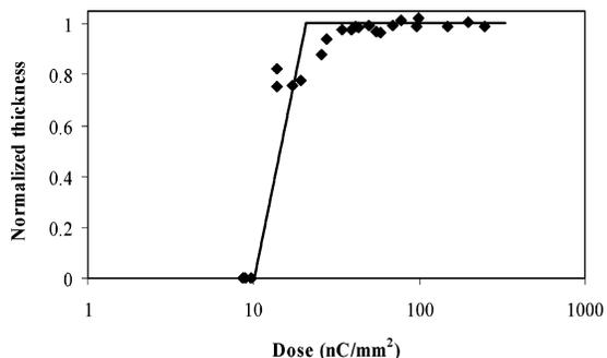
**Figure 1.** Contrast curve for 850 nm thick HSQ, exposed to 2 MeV protons. The straight line corresponds to a contrast of 3.2.
