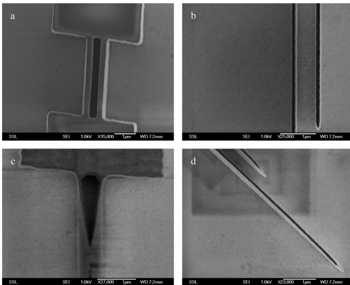
**Figure 2.** SEM images of parallel lines written with a 2 MeV  $\text{H}_2^+$  beam using a nine pixel wide exposure pattern in (a) 2  $\mu\text{m}$  thick SU-8 and 850 nm thick HSQ with (b)  $2.4 \times 10^6$  protons and (c)  $1.6 \times 10^6$  protons. In (d)  $2.0 \times 10^6$  protons are used in a seven pixel wide exposure pattern.
