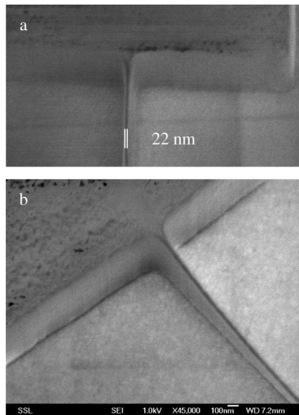
**Figure 3.** SEM images of a 22 nm wide line written with a 2 MeV H<sub>2</sub><sup>+</sup> beam using a three pixel wide exposure pattern in 850 nm thick HSQ with  $1.2 \times 10^6$  protons.
