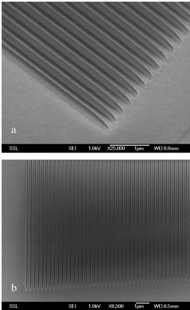
**Figure 4.** SEM images of a grating in 100 nm thick HSQ exposed with a 2 MeV  $H_2^+$  beam in an area of  $25 \times 50 \mu m^2$ .
