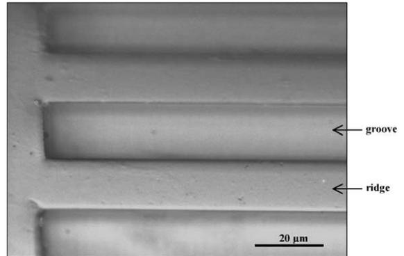
Fig. 2. Plan view of PMMA (2 mm thick) exposed by 1 MeV p-beam ( $1 \mu\text{m}$  spot size) and chemically developed.
