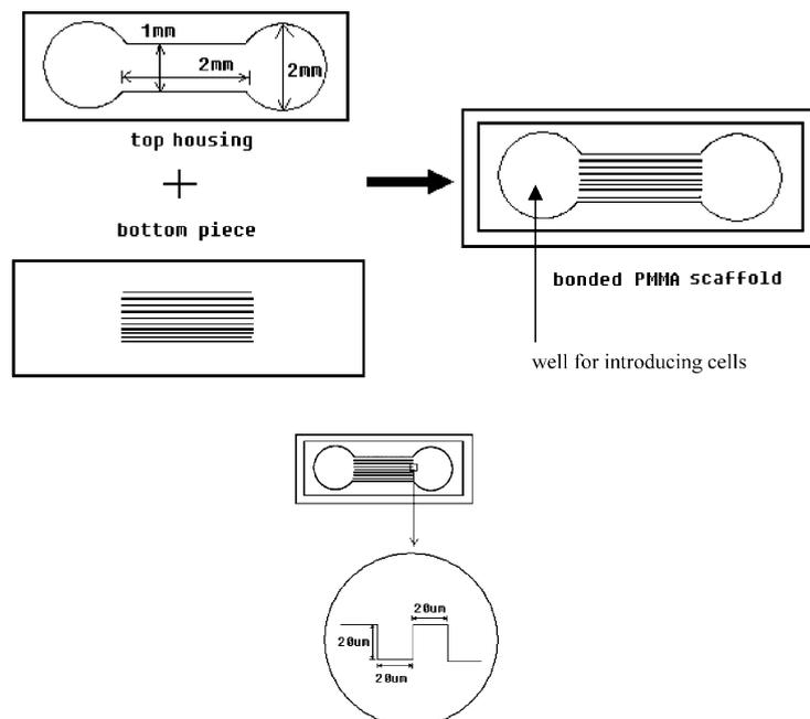
Fig. 3. Schematic representation of the fabrication process for bonding a top housing onto the 3D scaffold.
