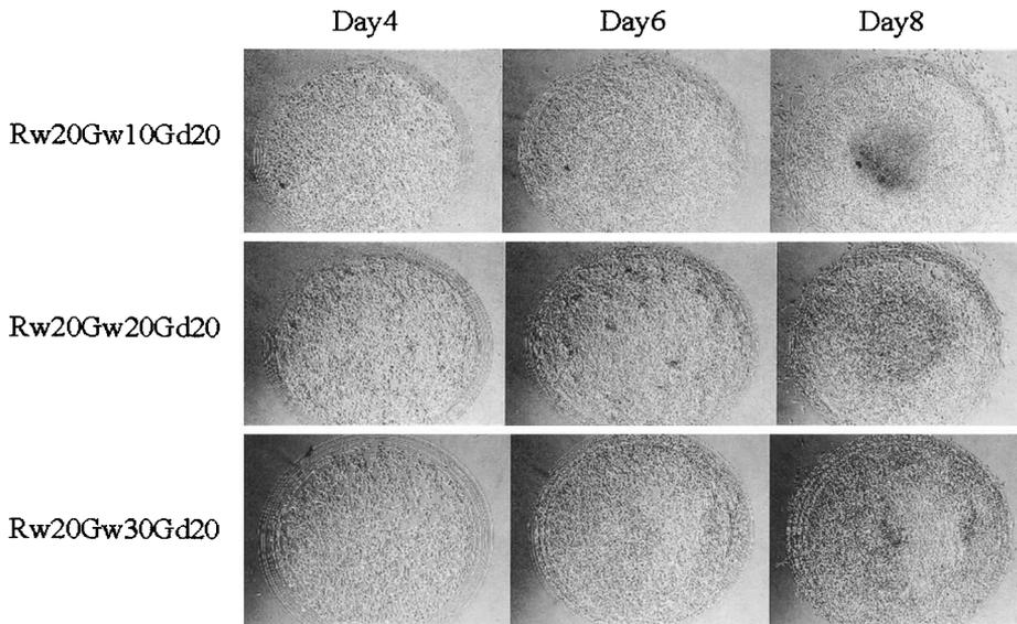
**FIG. 3.** Wider grooves are more effective in restricting fibroblasts. All dimensions are presented in micrometers. Rw, ridge width; Gw, groove width; Gd, groove depth. Day number indicates days after cell plating onto the central nonpatterned surface.
