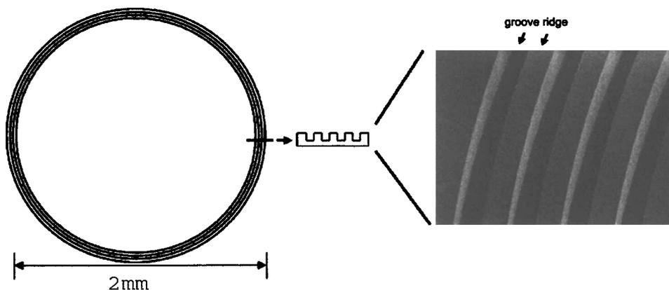
**FIG. 1.** A diagram of the 3D microstructure. The cross-section of the groove and ridge structure is shown in an amplified view. An SEM photo of the microstructure is also shown.
