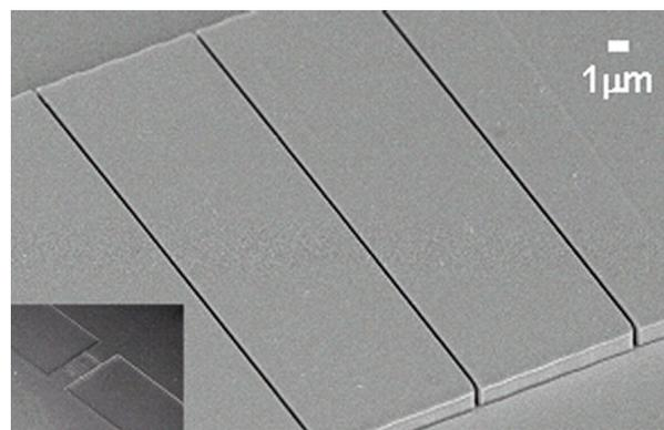
FIG. 3. Imprint of the Ni stamp in 8  $\mu\text{m}$  thick PMMA spin coated on a silicon substrate, showing reproducible fine features, smooth sidewalls, and vertical structures. Inset: low magnification view of the imprint.
