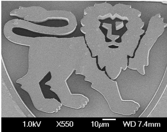
Fig. 4. Portion of the NUS logo micromachined on 30  $\mu\text{m}$  thick SU-8 on Si, within an area of 200  $\mu\text{m} \times 200 \mu\text{m}$  using photon normalization.
