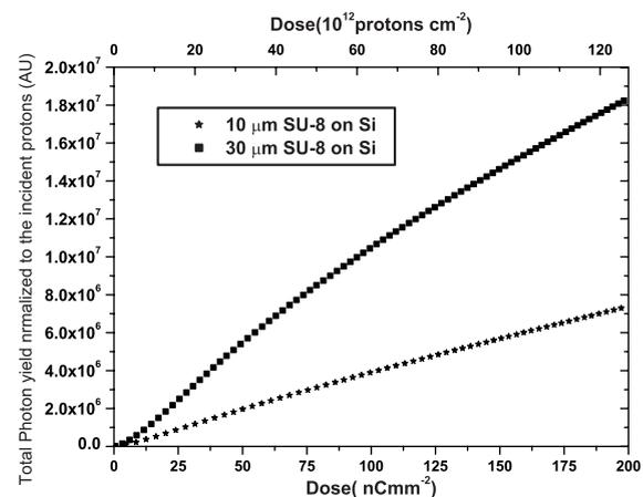
Fig. 3. Total photon yield normalized to incident protons versus dose.
