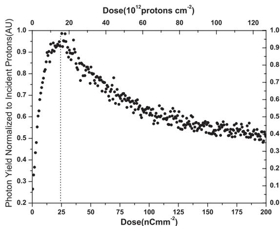
Fig. 2. Profile of photon yield from SU-8 normalized to the incident protons. The maximum photon yield per incident proton occur at  $25 \pm 5$  nC mm<sup>-2</sup>.
