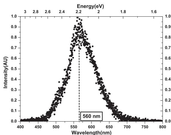
Fig. 1. 2 MeV proton induced luminescence spectrum of SU-8.
