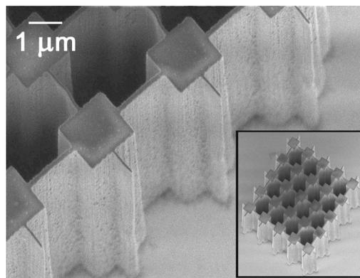
FIG. 2. SEM image of  $2 \times 2 \mu\text{m}^2$  pillars written in a  $10\text{-}\mu\text{m}$ -thick SU-8 layer (inset). Linking the pillars are high aspect ratio walls of width 60 and 120 nm. The structures were written with a 1 MeV proton beam.
