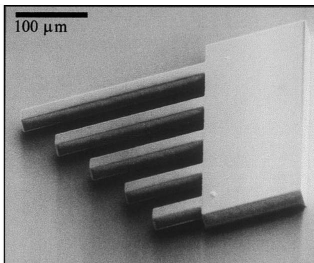
Fig. 2. SEM micrograph of a set of cantilevers produced in a  $36 \mu\text{m}$  thick SU-8 layer. The suspended cantilevers were produced using a 1.0 MeV proton exposure and the anchor was exposed using 2.0 MeV protons
