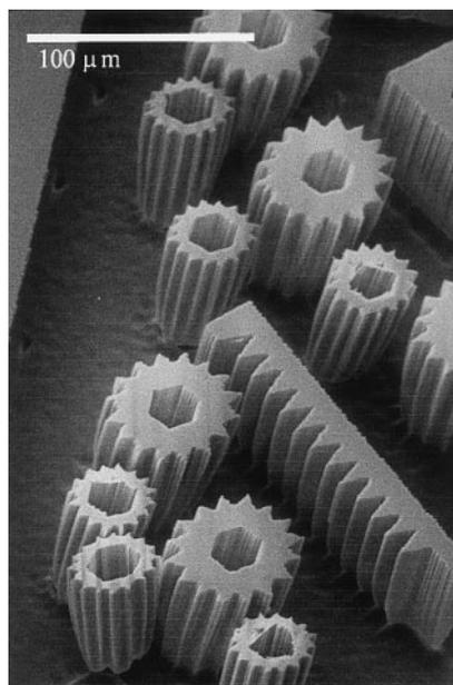
Fig. 1. SEM micrograph of cogs produced in bulk PMMA using a direct-write 2.0 MeV proton beam
