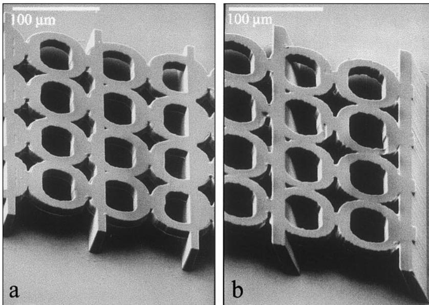
Fig. 4. SEM micrograph of self supporting circular structures anchored to a set of perpendicular (left) and 40° tilted (right) walls. A single 36  $\mu\text{m}$  thick layer of SU-8 resist was used in two exposures at proton energies of 0.6 MeV and 2.0 MeV
