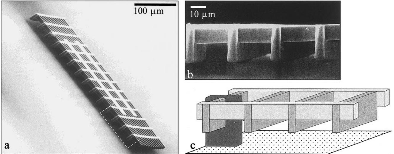
Fig. 3. SEM micrograph of a suspended multilevel grid produced in one 36  $\mu\text{m}$  thick layer of SU-8 resist using three exposures at proton energies of 0.6, 1.0 and 2.0 MeV
