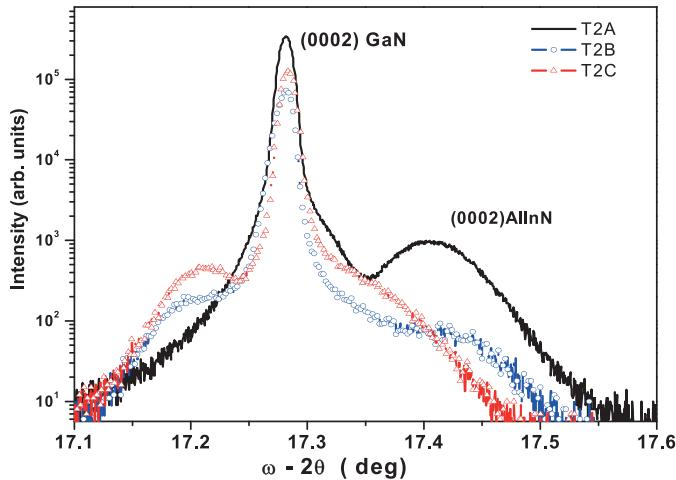
Figure 4. The (0002) HRXRD rocking curves of T2A, T2B and T2C samples. SHI-induced modification of strain in the epilayer is evident in spectra.
