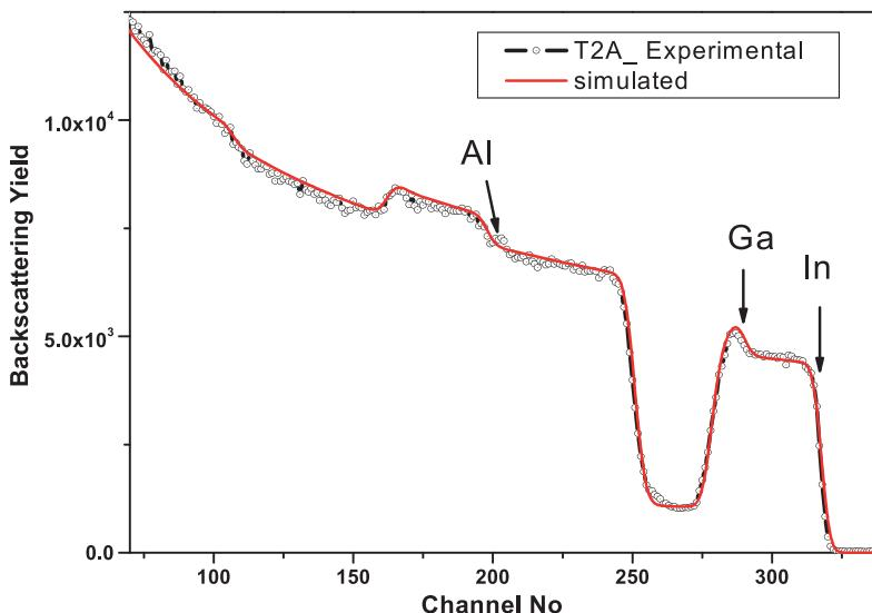
Figure 1. Measured and simulated RBS spectra of the T2A sample showing Ga diffusion into the indium energy window.
