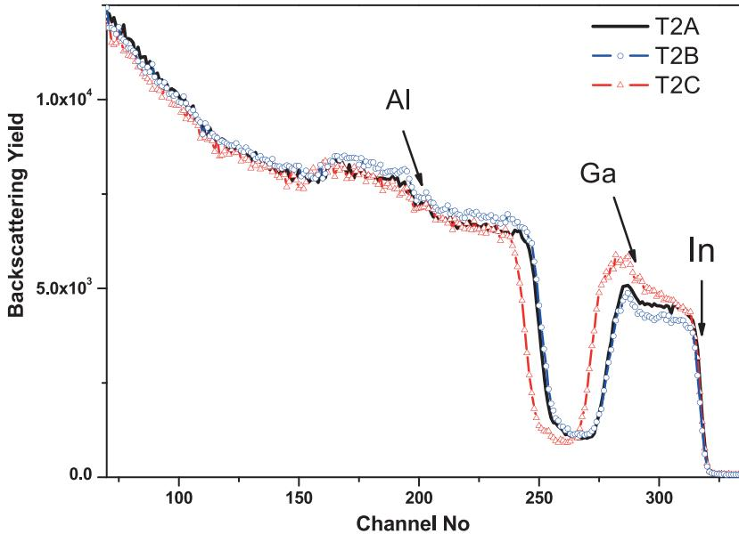
Figure 3. RBS spectra of T2A, T2B and T2C samples. SHI-induced diffusion of Ga from GaN into the AlInN epilayer is evident in spectra.
