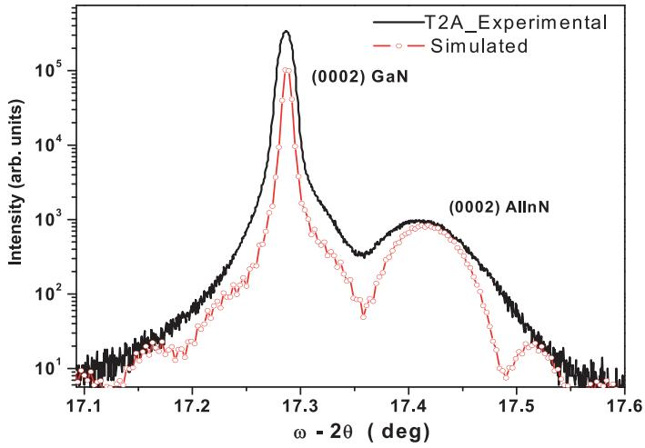
Figure 2. (0002)  $\omega - 2\theta$  X-ray diffraction for the T2A sample along with the theoretical simulated profile.
