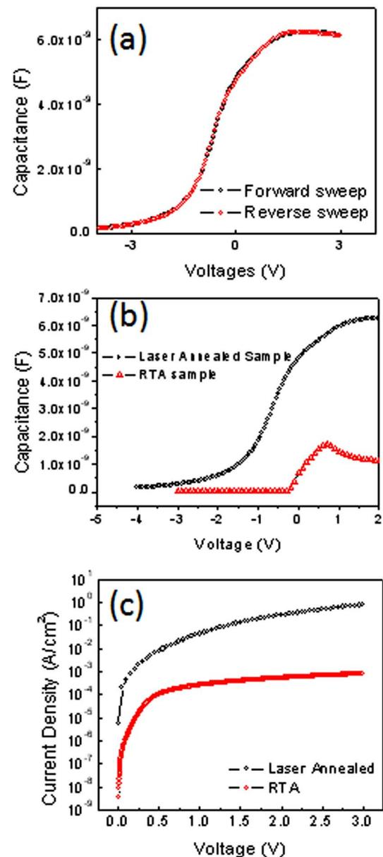
FIG. 3. (Color online) (a) High frequency (100 kHz) capacitance-voltage curve of  $\text{Au}/\text{Lu}_2\text{O}_3/n\text{-type Si}$  capacitors. (b)  $C$ - $V$  characteristic comparison between laser annealed and rapid thermal annealed samples. (c) Current density-voltage curve of  $\text{Au}/\text{Lu}_2\text{O}_3/n\text{-type Si}$  capacitors of laser annealed and rapid thermal annealed samples.
