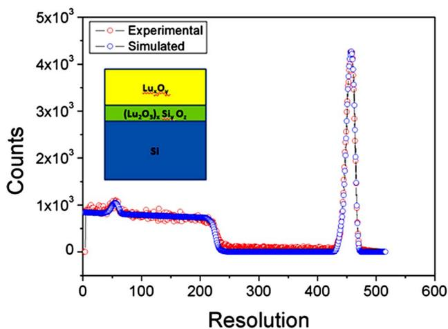
FIG. 2. (Color online) High-resolution RBS spectrum of  $\text{Lu}_2\text{O}_3/\text{Si}$  observed at scattering angle of  $65^\circ$ . The inset shows the simulated three-layer stack which corresponds closely to the observed HRTEM micrograph.
