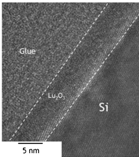
FIG. 1. Cross sectional HRTEM image of  $\text{Lu}_2\text{O}_3$  thin film after laser thermal irradiation showing an epitaxial behavior at the interface.
