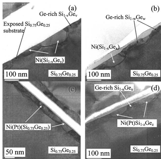
FIG. 4. Cross-sectional TEM micrographs of 10-nm Ni on Si<sub>0.75</sub>Ge<sub>0.25</sub> annealed at (a) 600 °C and (b) 700 °C and 10-nm Ni(Pt ~ 10 at. %) on Si<sub>0.75</sub>Ge<sub>0.25</sub> annealed at (c) 600 °C and (d) 700 °C, respectively. Here  $x < z < 0.25$  and  $w > u > 0.25$ .
