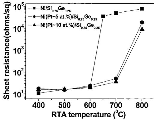
FIG. 1. Sheet resistance of 10-nm Ni, Ni(Pt~5 at. %), and Ni(Pt~10 at. %) on Si<sub>0.75</sub>Ge<sub>0.25</sub> after various RTA temperatures.
