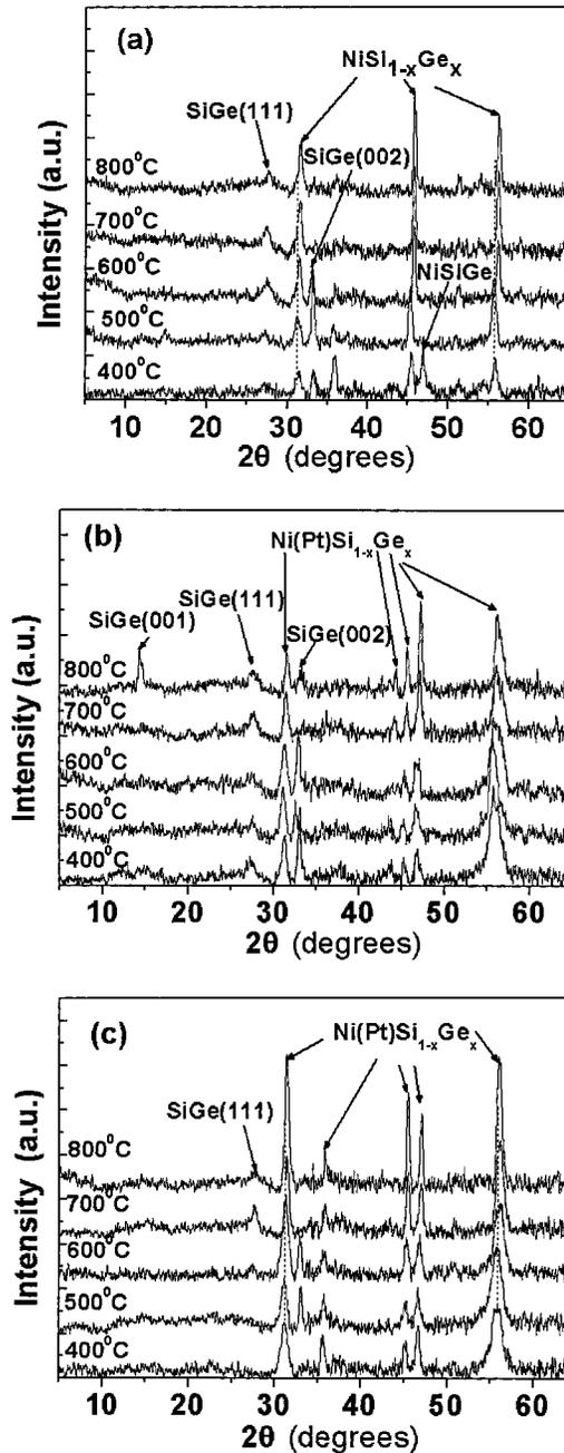
FIG. 2. XRD of 10-nm (a) Ni, (b) Ni(Pt~5 at. %), and (c) Ni(Pt~10 at. %) on Si<sub>0.75</sub>Ge<sub>0.25</sub> annealed at different RTA temperatures.
