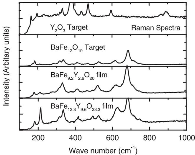
FIGURE 3 The Raman spectra of BaFe<sub>12.3</sub>Y<sub>9.6</sub>O<sub>33.3</sub> and BaFe<sub>9.2</sub>Y<sub>2.6</sub>O<sub>20</sub> materials as well as Y<sub>2</sub>O<sub>3</sub> and BaFe<sub>12</sub>O<sub>19</sub> targets
