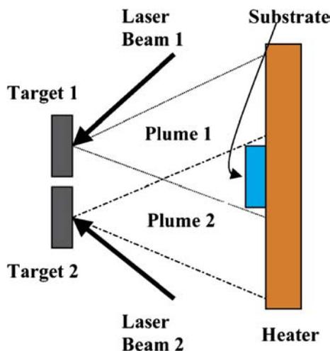
FIGURE 1 The schematic diagram of the laser synthesis system
