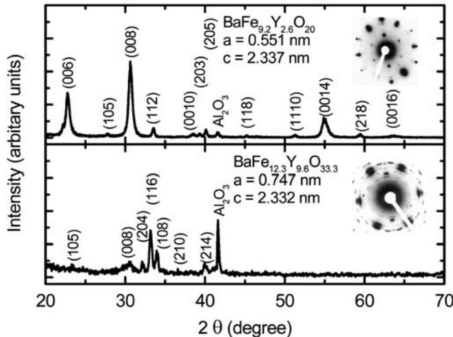
FIGURE 4 The XRD data and selected area diffraction patterns of BaFe<sub>12.3</sub>Y<sub>9.6</sub>O<sub>33.3</sub> and BaFe<sub>9.2</sub>Y<sub>2.6</sub>O<sub>20</sub> materials on single-crystal Al<sub>2</sub>O<sub>3</sub> substrates
