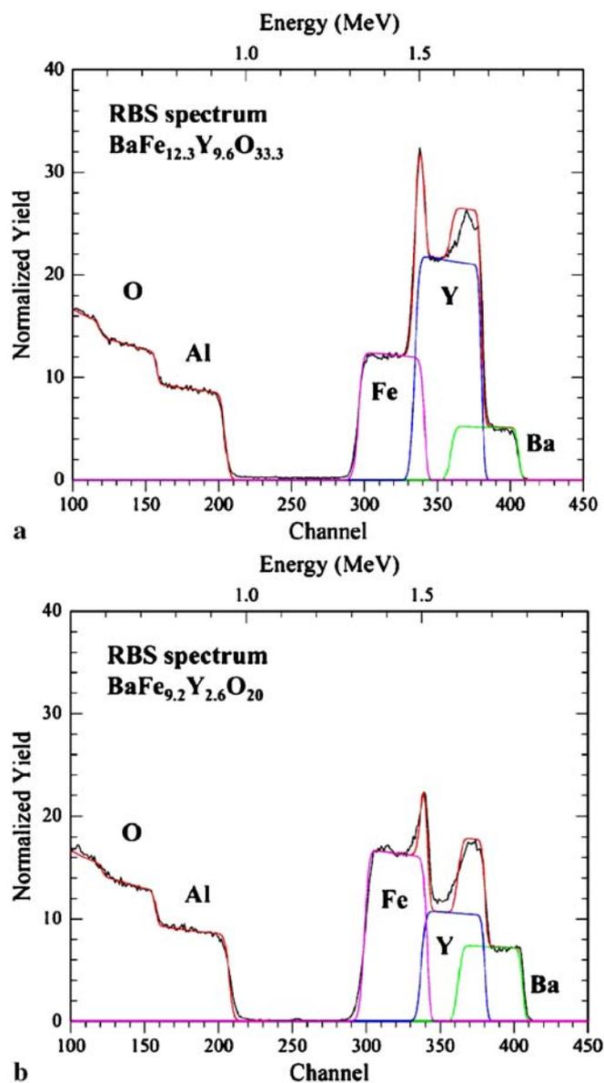
FIGURE 2 The RBS spectra of  $\text{BaFe}_{12.3}\text{Y}_{9.6}\text{O}_{33.3}$  and  $\text{BaFe}_{9.2}\text{Y}_{2.6}\text{O}_{20}$  materials on single-crystal  $\text{Al}_2\text{O}_3$  substrates
