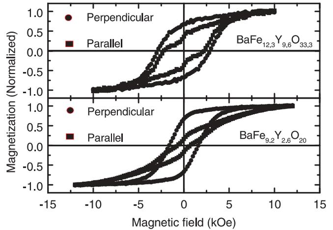
FIGURE 5 The magnetization hysteresis loops of BaFe<sub>12.3</sub>Y<sub>9.6</sub>O<sub>33.3</sub> and BaFe<sub>9.2</sub>Y<sub>2.6</sub>O<sub>20</sub> materials on single-crystal Al<sub>2</sub>O<sub>3</sub> substrates
