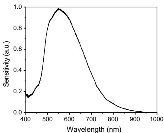
Fig. 2. Sensitivity curve of the Ocean Optics USB2000 spectrometer and light collection system.
