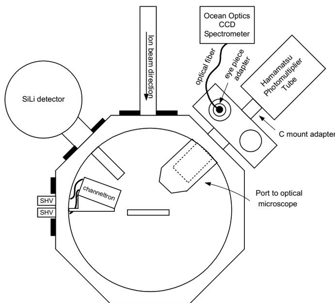
Fig. 1. Schematic diagram of simultaneous IL and IBISE setup.
