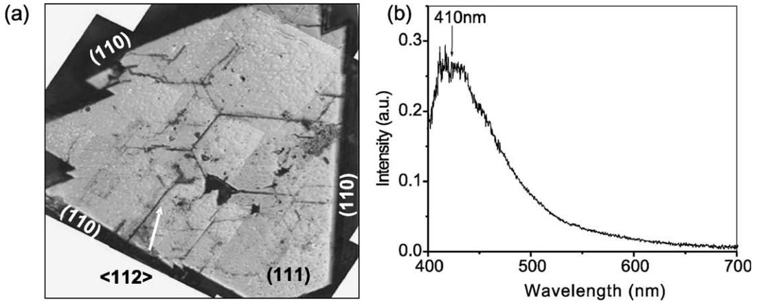
Fig. 3. (a) Nomarski optical micrograph and (b) IL spectrum of Al-doped c-BN sample.
