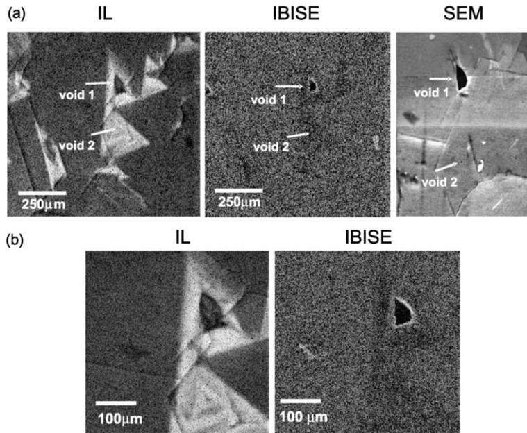
Fig. 4. (a) Panchromatic IL and IBISE images collected over an area of  $1 \times 1 \text{ mm}$ , and SEM micrograph showing void 1 and 2. (b) IL and IBISE images over an area of  $400 \times 400 \mu\text{m}$  about the central area in (a).
