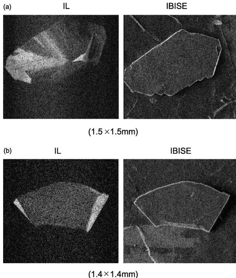
Fig. 5. IL and IBISE images of two grains of undoped (100) c-BN.
