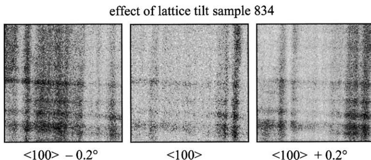
Fig. 6. CCM maps from sample 834, plotted is region 2 (see Fig. 5). Shown are maps generated with  $\langle 100 \rangle$  alignment and with the sample rotated by  $\pm 0.2$  along the  $(010)$  planar direction.
