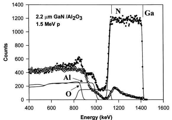
Fig. 1. Random and [000 1] channelled 1.5 MeV H<sup>+</sup> backscattering spectra from a 2.2 μm GaN/Al<sub>2</sub>O<sub>3</sub> sample, together with the deconvolution of the signals from the elements present. For Ga and N the surface energies are indicated.
