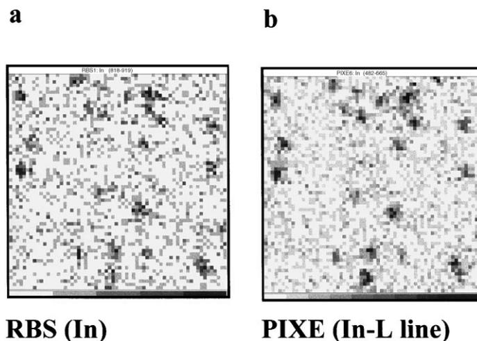
Fig. 6. Two MeV  $\text{He}^+$  backscattering CCM maps the sample described in Fig. 5. (a) The integral of the In backscattering signal is mapped. (b) The In-L X-ray intensity is mapped. The gray-scale indicates intensity, darker regions have higher intensities.
