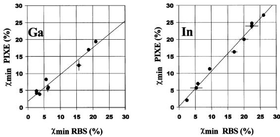
Fig. 7. Comparison of the PIXE and RBS channeling yields measured for Ga and In from nine InGaN/GaN samples.
