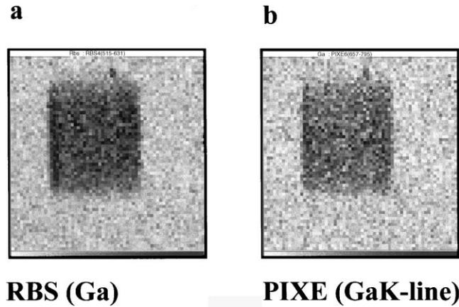
Fig. 2. 1.5 MeV H<sup>+</sup> backscattering CCM maps from the random implant. (a) The integral of the Ga backscattering signal is mapped. (b) The Ga–K intensity is mapped. The gray-scale indicates intensity, darker regions have higher intensities.
