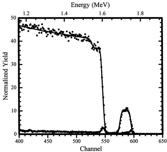
Fig. 5. Random and [0001] channelled 2 MeV  $\text{He}^+$  backscattering spectra from 500 Å  $\text{In}_{0.11}\text{Ga}_{0.89}\text{N}/\text{GaN}$ .
