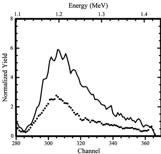
Fig. 3. The Ga-region in the channeled 1.5 MeV H<sup>+</sup> backscattering spectra from damaged (full line) and undamaged (dotted line) regions of the map in Fig. 2(a).
