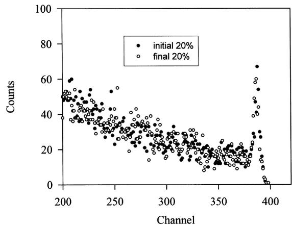
Fig. 4. One MeV He<sup>+</sup> [000 1] channeled spectra taken during the  $7.4 \times 10^{16}$  He<sup>+</sup>/cm<sup>2</sup> channeled implant. Spectra taken during the initial 20% and the final 20% of the irradiation are shown.
