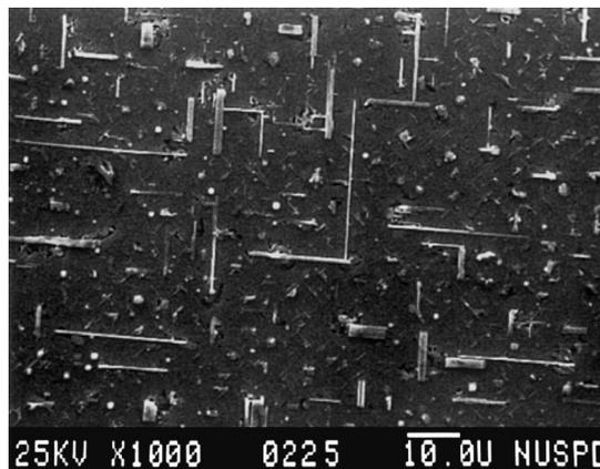
Fig. 1. SEM image of an Ag-doped YBCO sample.
