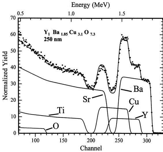
Fig. 2. RBS spectrum of an undoped YBCO/SrTiO<sub>3</sub> sample, the contributions from the individual elements are indicated.
