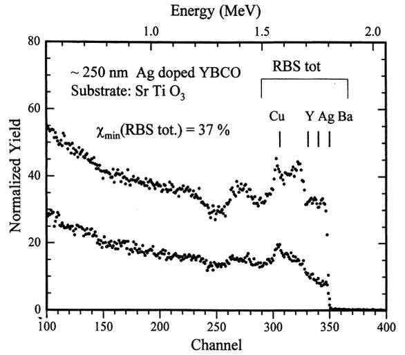
Fig. 3. Random and channeled RBS spectra from an Ag-doped YBCO sample. The surface energies of the metals in the film are indicated.
