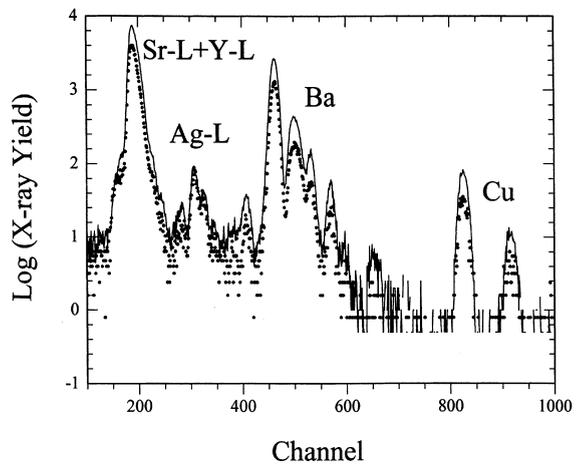
Fig. 4. PIXE spectra taken simultaneously with the RBS data from Fig. 3. The fully drawn line indicates the random spectrum, and the dotted line shows the aligned spectrum.
