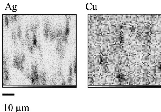
Fig. 5. PIXE elemental maps for Ag and Cu taken from an Ag-doped YBCO sample.
