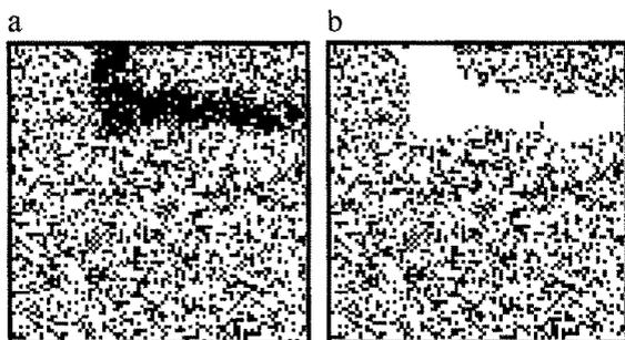
Fig. 1. (a) Elemental Fe map of Mong Hsu ruby showing Fe surface contamination in the upper right. Scan size was 200  $\mu\text{m}$ . (b) Part of the map from (a) that is used to generate the PIXE spectrum.
