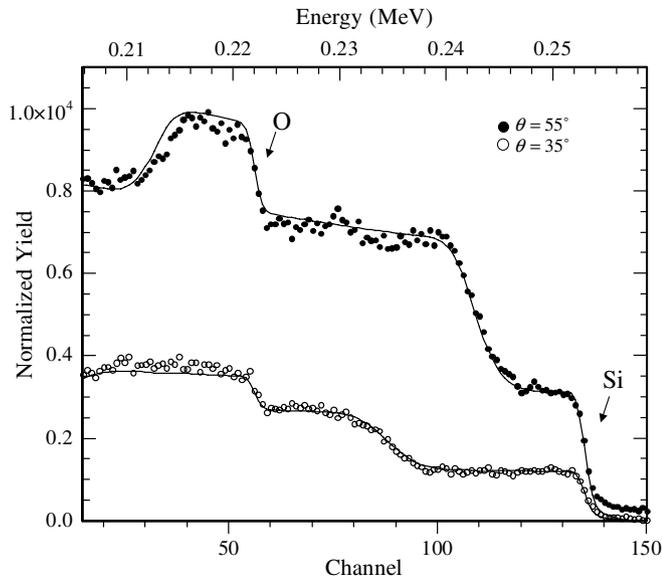
Fig. 4. HRBS spectra of 10 nm SiO<sub>2</sub>/Si, the full lines are RUMP simulations. The Si and O surface edges are indicated.
