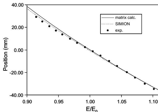
Fig. 3. Comparison of leading edge positions with calculations from matrix theory and the SIMION simulation code.
