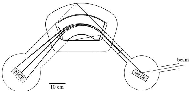
Fig. 1. Sketch of the CIBA high resolution RBS endstation, the median plane trajectories of particles with  $\varepsilon = E/E_0 = 0.88$ , 1 and 1.15 are indicated.
