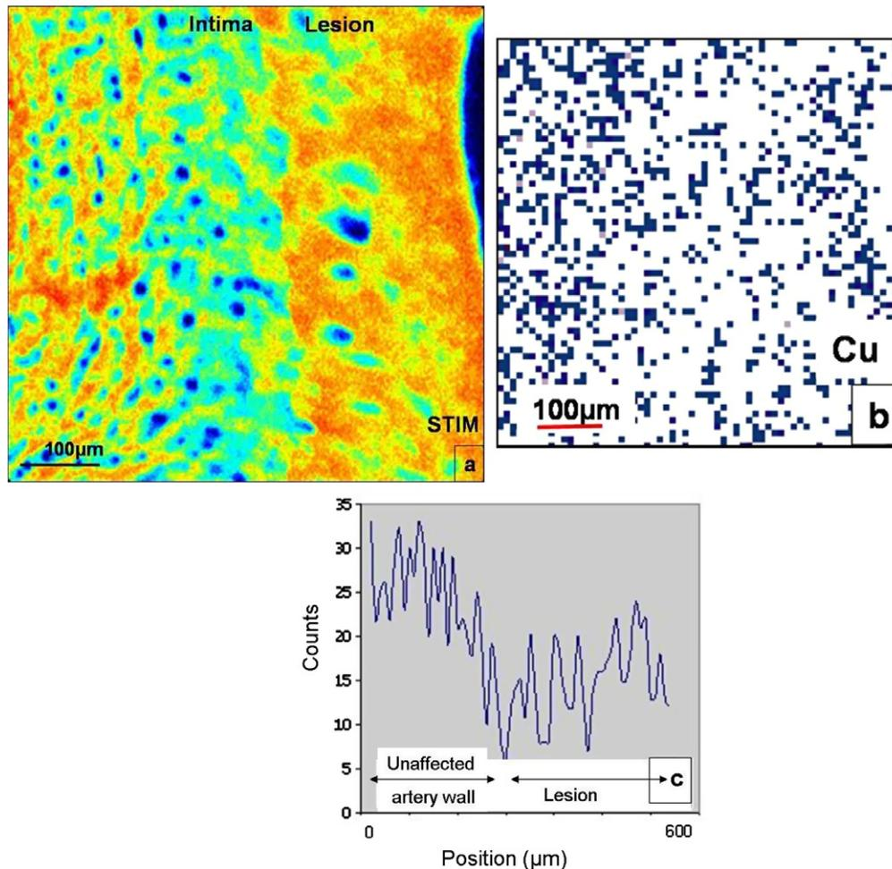
Fig. 1. Atherosclerosis in the cholesterol-fed rabbit. (a) STIM image of part of an artery cross section, showing unaffected artery wall + lesion, (b) representative copper map, of the area, and (c) copper X-ray (PIXE) counts represented as a line scan from right to left across the unaffected wall and lesion. Elemental data extracted from (b) and (c) show that in this sample the average copper concentration is 2.7 ppm in the lesion and 7.4 ppm in the healthy artery wall.
